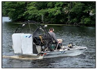
for on-board mixing of liquid product, which is then injected into the water column. This methodology helps get the herbicide down to the plants where they are most susceptible to concentrations of herbicide.
