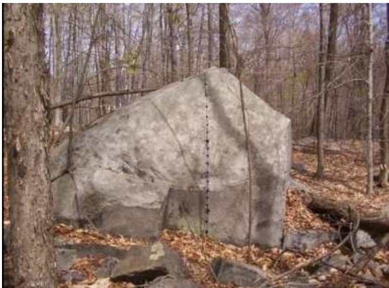
Boulder with drill holes demonstrating the “boulder quarrying” method of hand cutting stone slabs.
